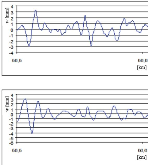
Fig. 5. An excerpt from track twist measurement results [mm/m] provided by a recording coach travelling along approx. 100 m of a railway line track with a maximum velocity of 200 km/h
