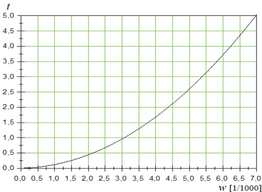
Fig. 4. Relationship between track twist  $w$  and its conversion value
