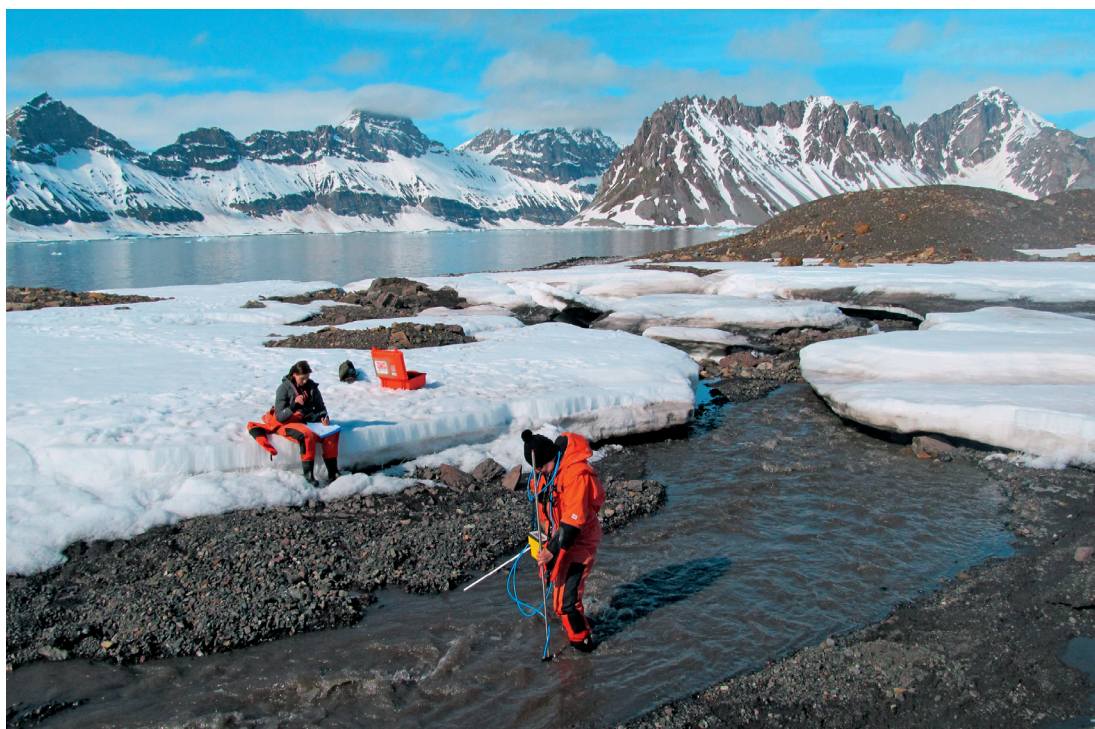
Measuring water flow in the river Lorschelv
