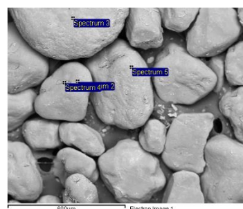
Fig. 15. Spots where the chemical composition was analyzed for moulding sand after the ablation process
