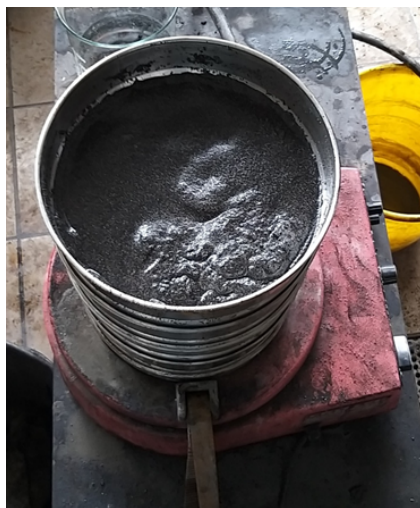
Fig. 4. Wet separation with use of the vibrating classifier
