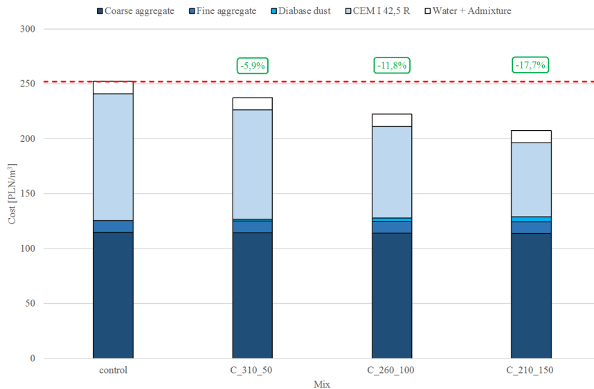
Fig. 7. The estimation of the cost of the concrete mix with various diabase dust content
