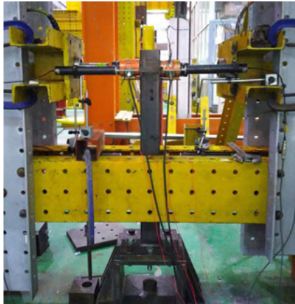
(a) Test setup without axial load
