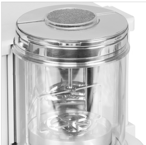
Fig. 8. Balance during the measurement of magnetic susceptibility.
