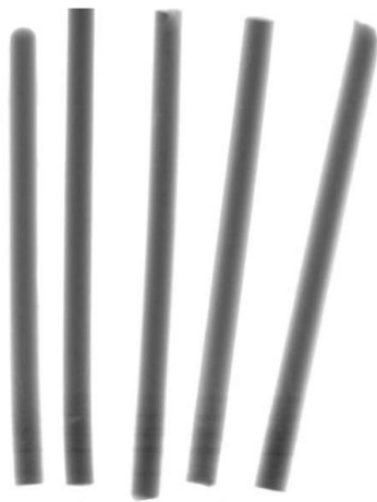
Fig. 4. X-ray images of tensile test bars
