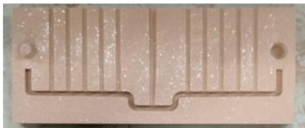
Fig. 2. Sand moulds for producing 10 tensile test bars
