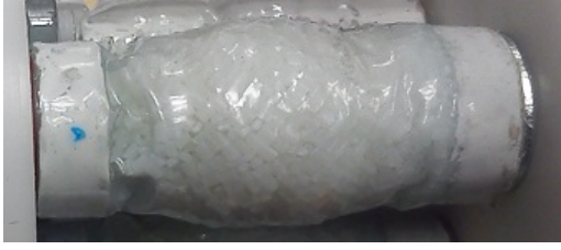
Fig. 4. VPP damper filled with polystyrene
