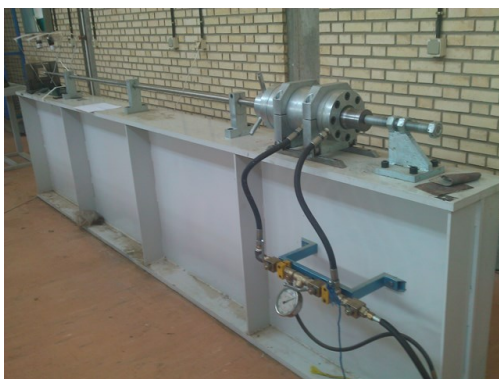
Fig. 1. Gas gun used for performing ballistic tests
