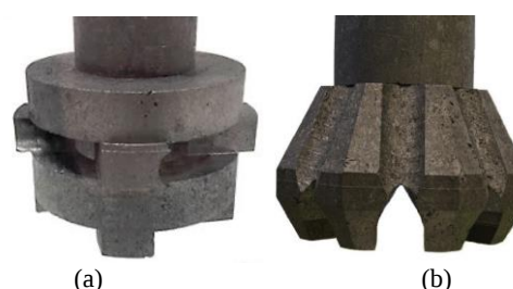
Fig. 3. The impeller variants: (a) F2A 190, (b) J8 190
