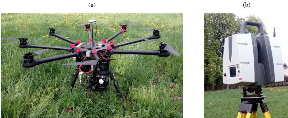
Fig. 1. Measuring equipment used: a) UAV – DJI S1000, b) TLS – Leica P40 ScanStation
