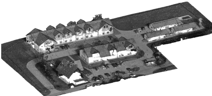
Fig. 5. Point cloud – derived from UAV photos
