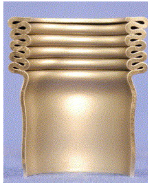
Fig. 1. Axisymmetric mode of deformation [1]
