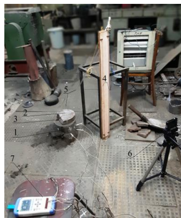
Fig. 4. General view of the set up used in the experiment to study pressure changes in the centre of the spherical casting: 1 - casting mold; 2 - load; 3 - funnel for pouring metal; 4 - U-shaped water manometer; 5 - silicone tube connecting the manometer to the needle; 6 - video recording of manometer readings; 7 - AE4808 device for temperature measuring
