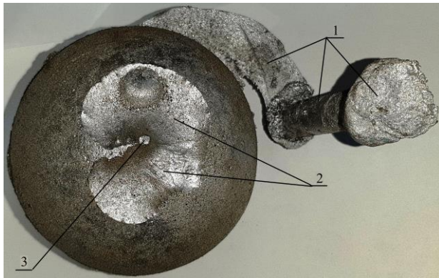
Fig. 7. Top view of the casting ball \varnothing 120 mm with the gating system (1), shrinkage depression (2) and remnant of an air gate (3)
