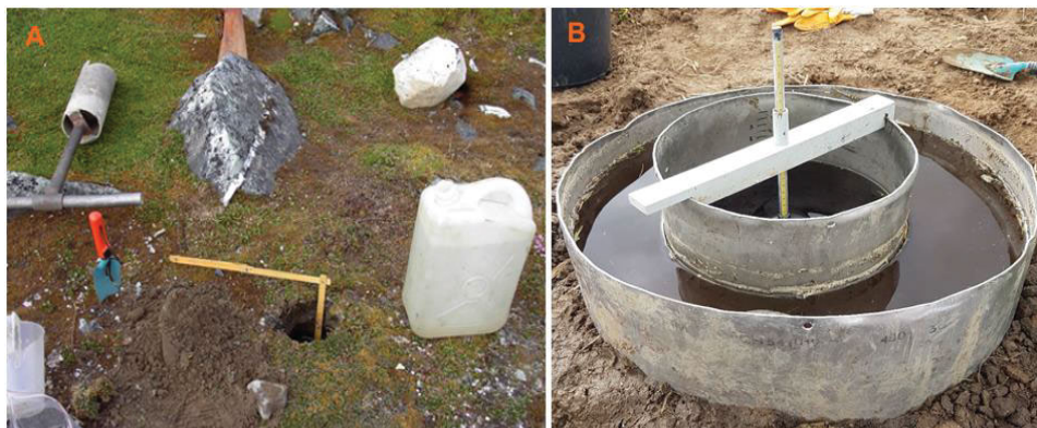
Fig. 3. Field measurement of sediment permeability using Porschet method (A) and the Eijkelkamp double-ring infiltrometer (B).
