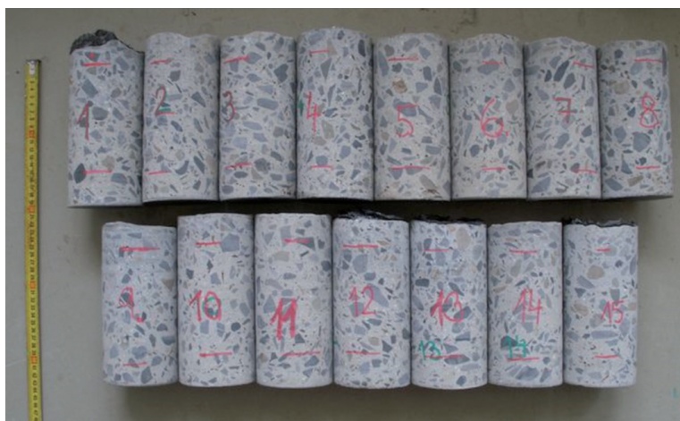
Fig. 5. Laboratory samples from the industrial floor of the production hall in Ostrava–Vítkovice
