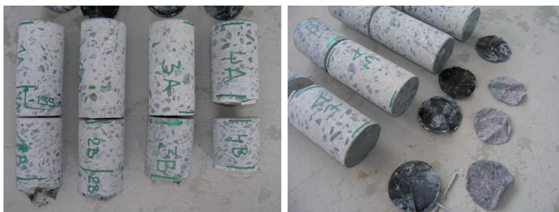
Fig. 7. Laboratory samples from the industrial floor of the storage hall in Frýdek–Místek
