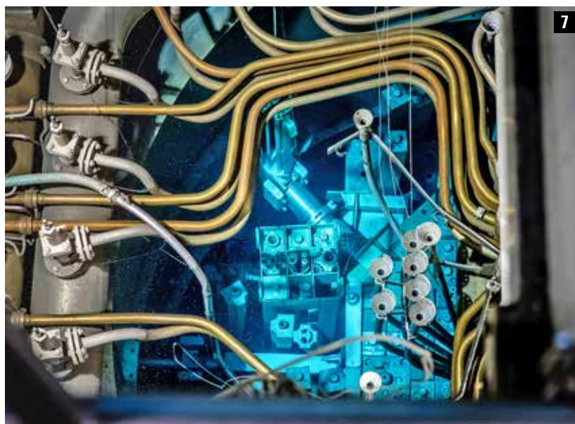
Photo 6 Manipulator pulling the ISHTAR high-temperature capsule into the hot cell
