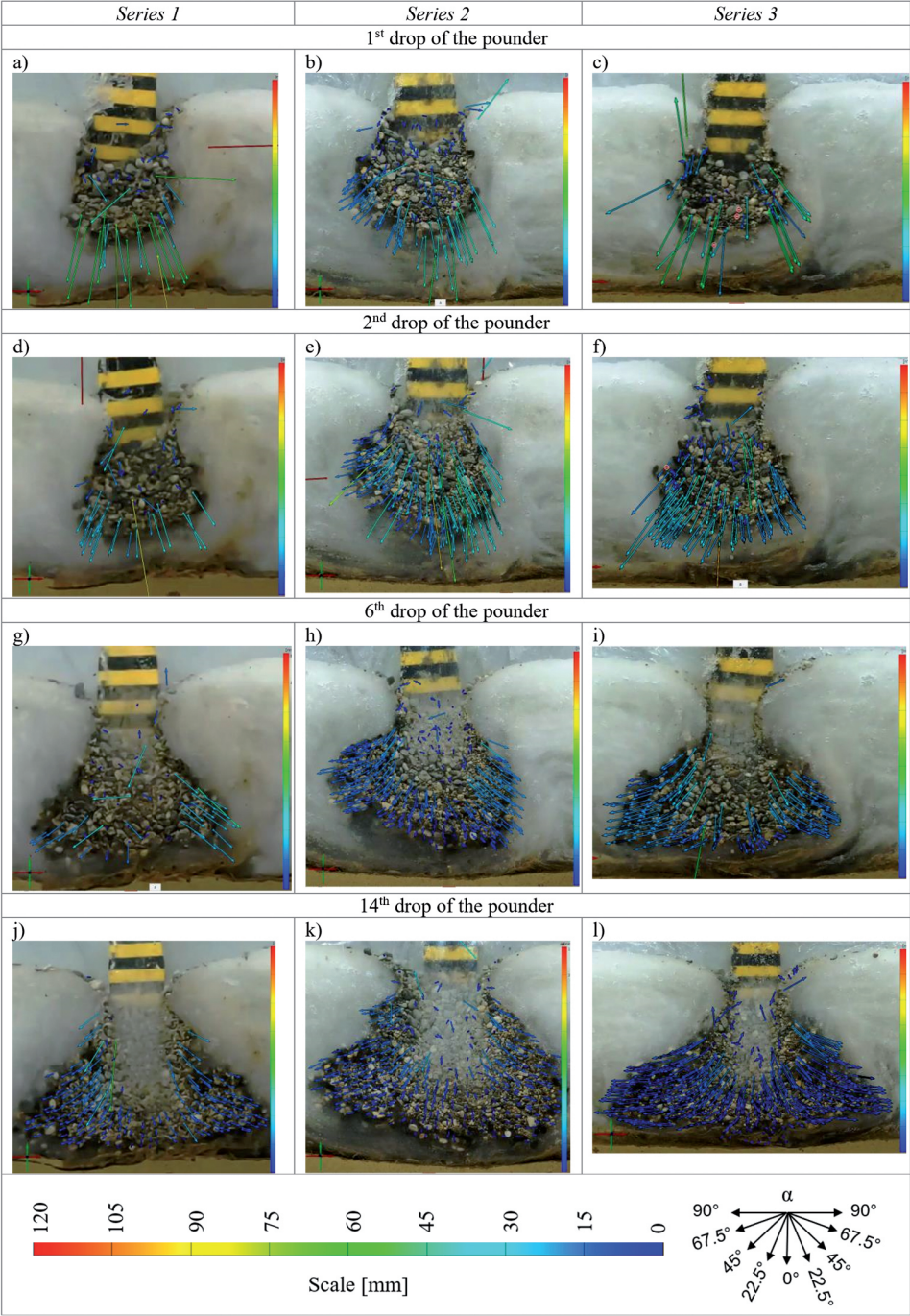
Fig. 8. The vectors of the resultant displacements of the backfill material – column C, H_s/H_p = 1.5
