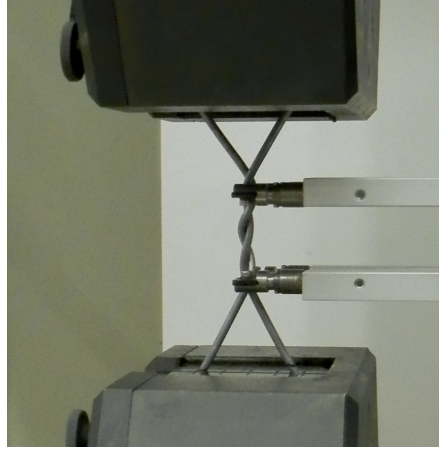
Fig. 8. Double twist during testing
