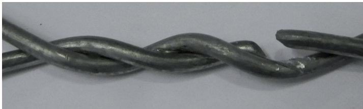
Fig. 9. Double twist after failure
