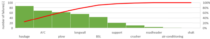
Fig. 16. Pareto chart for the number of electrical failures in plow longwalls
