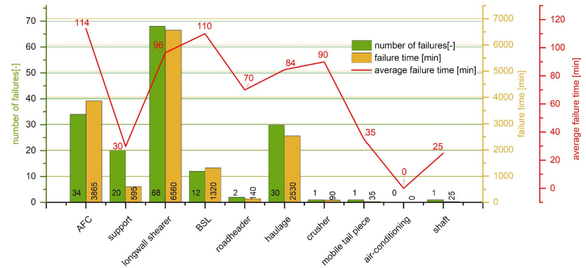
Fig. 9. Number, duration and average duration of mechanical failures in shearer longwalls
