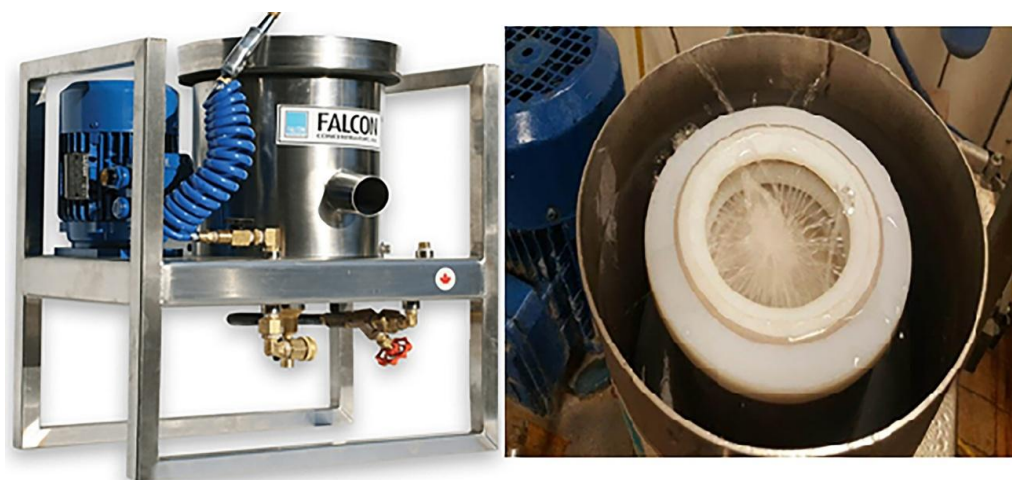
Fig. 2. Falcon L40 concentrator and top view of the concentrator bowl
