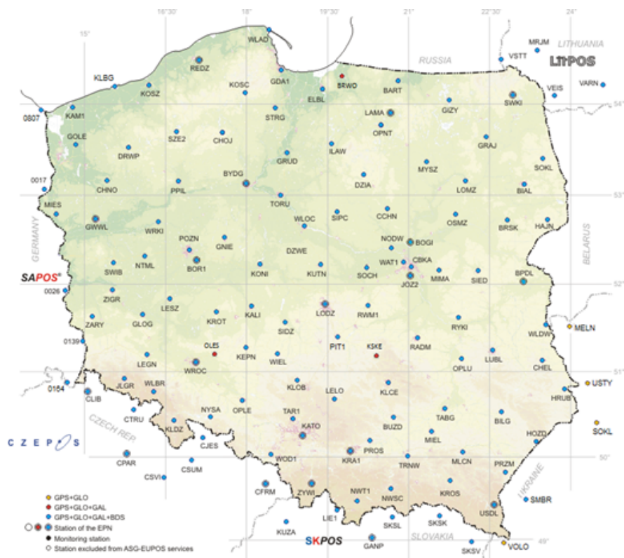
Fig. 6. Reference stations of the ASG-EUPOS system (as of February 2023, www.asgeupos.pl )
