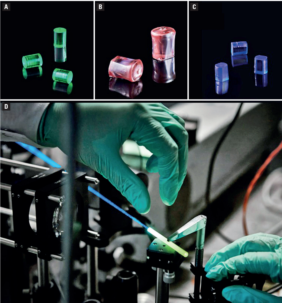
Crystals grown by members of the E3 staff: (A) yttrium-aluminum garnet doped with praseodymium YAG:Pr (used in scintillation techniques), (B) yttrium orthovanadate doped with neodymium YVO 4 :Nd (used in the construction of lasers), (C) magnesium spinel doped with cobalt MgAl 2 O 4 :Co (used in the construction of lasers), (D) optical work underway in the E3 optics laboratory
