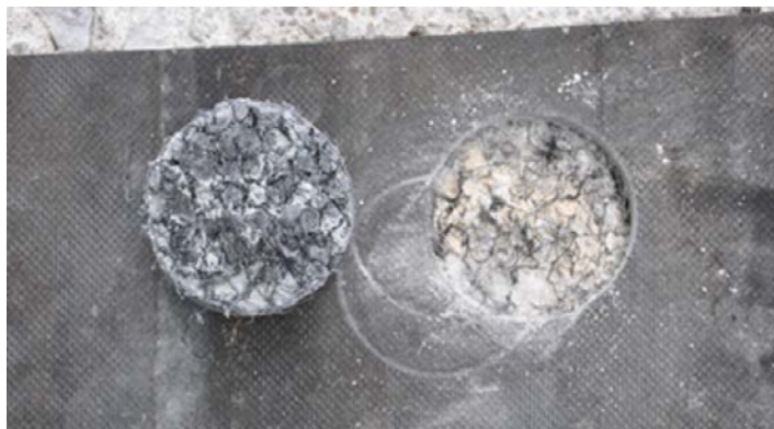
Fig. 10. Failure between the plastic hook-and-loop-like anchor layer and the concrete surface of the sleeper (failure type A/B)
