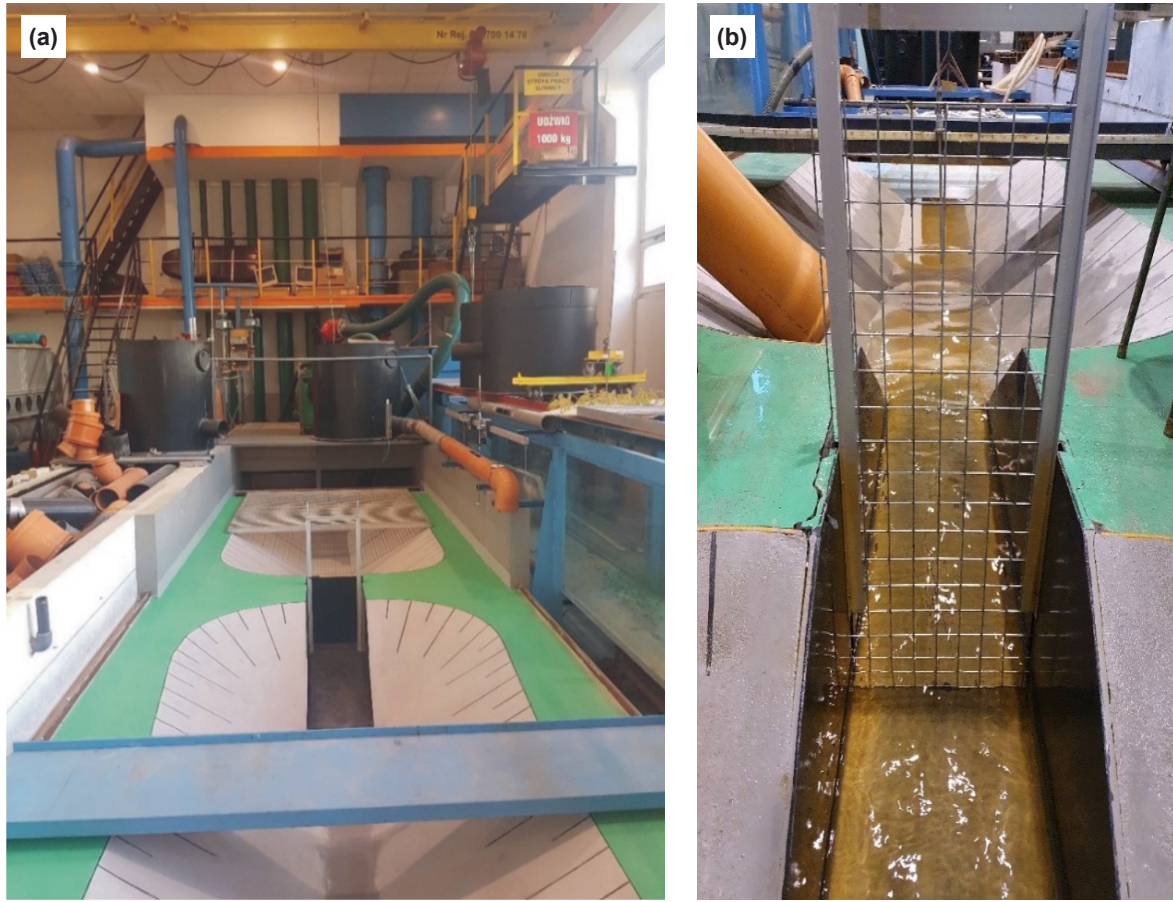
Figure 2. The sluice gate (a) used in the 1 experimental case and trash racks (b) in the 2 case, mounted in vertical guides
