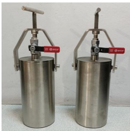
Fig. 2. Hermetically sealed containers for coal sampling
