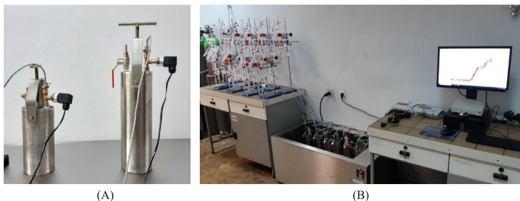
Fig. 3. Central Mining Institute – National Research Institute test stand for methane content determination by the USBM direct method: (A) hermetically sealed containers with pressure and temperature sensors; (B) the original measurement system
