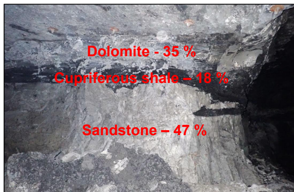
Fig. 3. An example of copper deposit structure in the SI-XII field, the “Polkowice-Sieroszowice” copper ore mine
