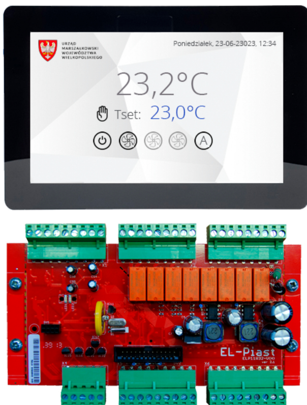
Fig. 11. A set of room automation devices designed for measuring, setting the temperature and regulating the operation of the air handling unit. The PLC controller is located in the power supply and control cabinet together with other automation components necessary for the operation of air conditioning and ventilation. The operator panel is located on the wall of the rooms
