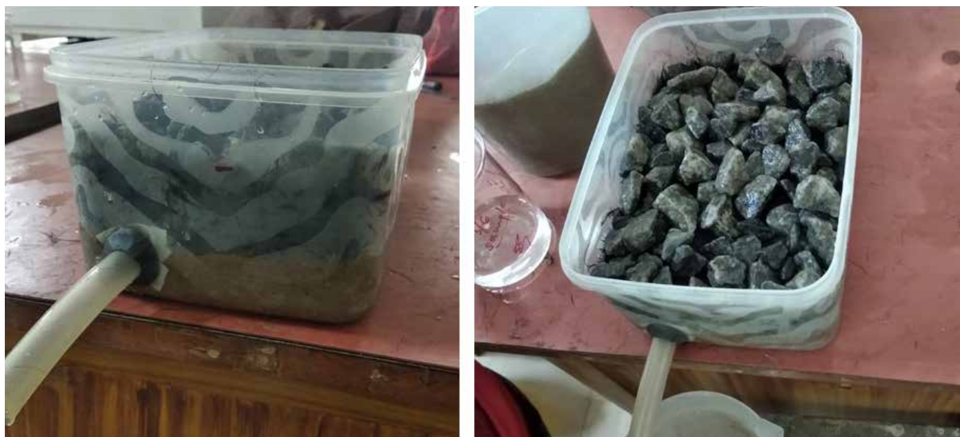
Fig 1. Constructed wetland for pilot study (An image showing the plastic box in which the layers of sand, adsorbent-hair, and gravel is filled to perform the experiment)
