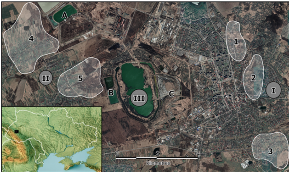
Fig. 1. The Kalush–Holyn deposit. Mines: I – Kalush, II – Nova Holyn, III – Dombrovsky quarry; mine fields: 1 – Northern kainite field, 2 – Central kainite field, 3 – Khotin sylvinite field, 4 – Eastern Holyn field, 5 – Sivka-Kalush: A – tailings, B – accumulating basins, C – quarry dumps
