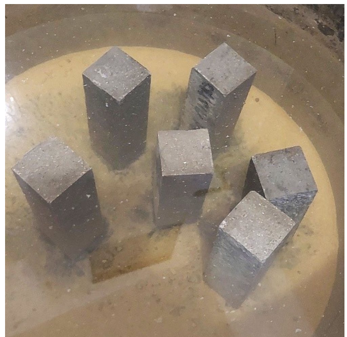
Fig. 7. The water absorption test
