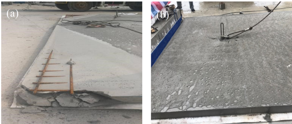
Fig. 8. Surface quality of SCC filling layer: (a) 170 \text{ kg/m}^3 ; (b) 182 \text{ kg/m}^3
