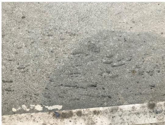
Fig. 12. Effect of 54% sand ratio on the quality of filling layer
