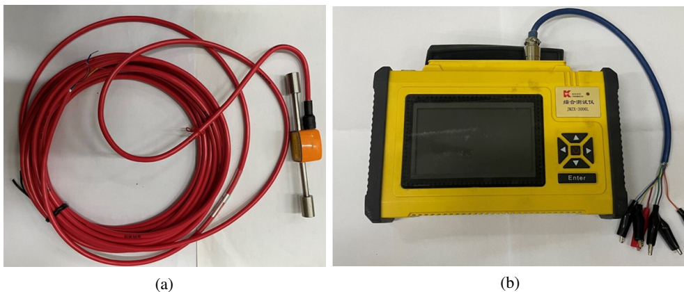
Fig. 3. Monitoring equipment: (a) Strain sensor; (b) Portable comprehensive tester
