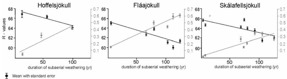
Text-fig. 9. Change in Schmidt hammer R-values and weathering rind thickness versus duration of weathering on forelands of Hoffellsjökull, Fláajökull and Skálafellsjökull
