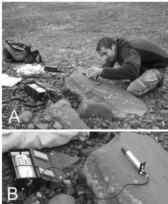
Text-fig. 3. Measuring rock surface micro-roughness of glacially-abraded boulder (A); Handysurf E35-B profilometer (B). Phot. A.Tittenbrun
