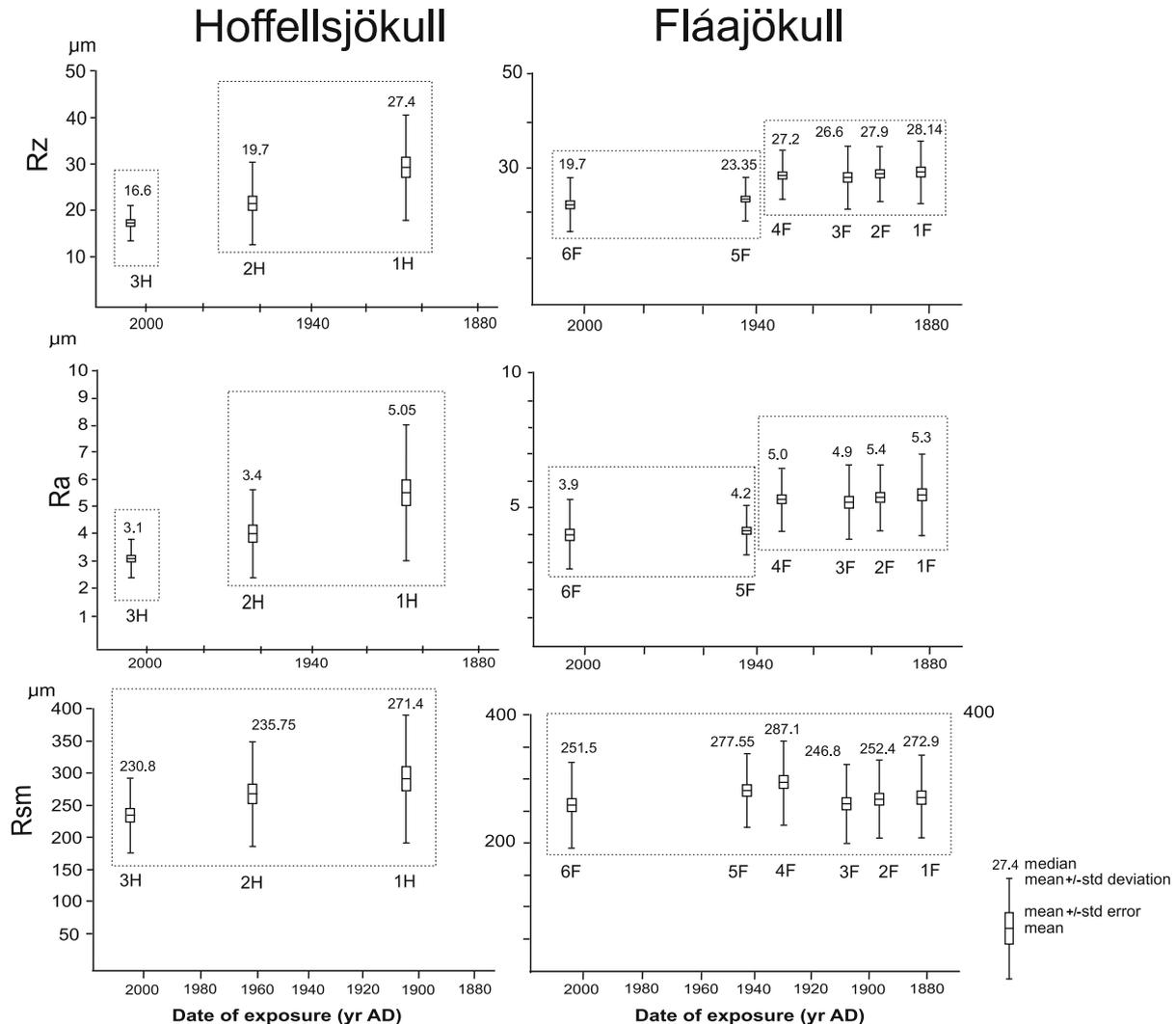
Text-fig. 5. Micro-roughness change on test sites within forelands of Hoffellsjökull and Fláajökull; large dotted rectangles include populations of readings which do not significantly differ from each other according to Kruskal-Wallis and multiple comparison post-hoc tests
