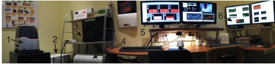
Fig. 6. The view of the measurement system: 1 – scanning head, 2 – PXI unit, 3 – personal computer with AFM measurement software and LabView 2010 programming environment, 4 – AFM controller, 5 – AFM measurement software, 6 – developed software working simultaneously
