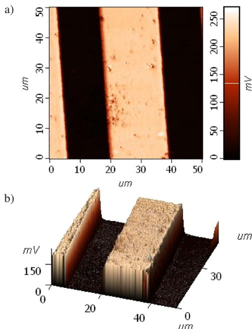
Fig. 4. Sensor structure obtained by means of the confocal microscopy method (the dark spaces – graphene on a glass surface, the brighter spaces – graphene on a gold interdigital electrode)
