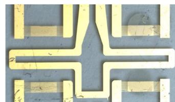
Fig. 1. Sensing structure with 4 resistance interdigital electrode structures
