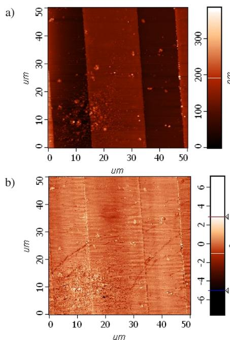
Fig. 3. AFM image of the surface of the electrode structure: a) amplitude image; b) phase image; (the dark spaces in Fig. 3a present graphene on a glass surface, the brighter spaces – graphene on a gold interdigital electrode)
