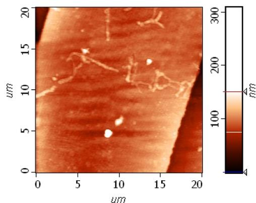
Fig. 20. AFM phase image of the surface of the electrode structure with graphene after numerous cycles of deposition of the synthetic air with  $\text{NO}_2$  and steam
