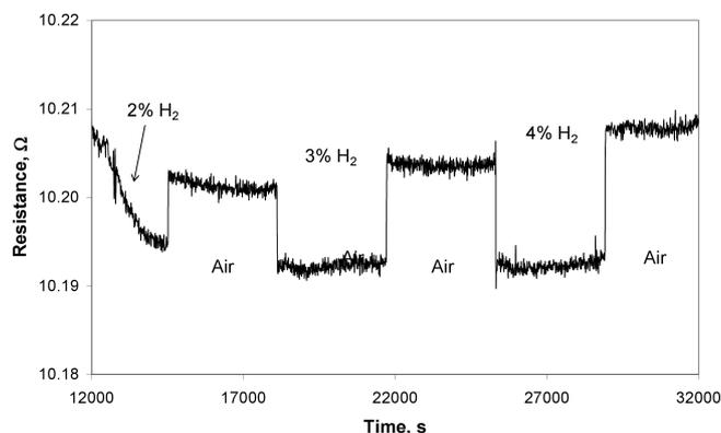
Fig. 14. Sensitivity of a resistance graphene structure with a 3nm layer of Pd to the presence of H<sub>2</sub> in an atmosphere of synthetic air (temperature 50°C)
