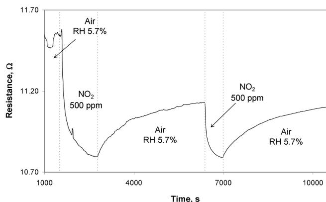
Fig. 17. Sensitivity of the sensor structure with graphene to the presence of  $\text{NO}_2$  in the atmosphere of synthetic air (temperature of the structure  $120^\circ\text{C}$ , humidity RH about 5%)
