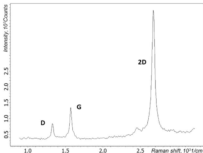
Fig. 5. Raman's spectrum of graphene on the sensor structure
