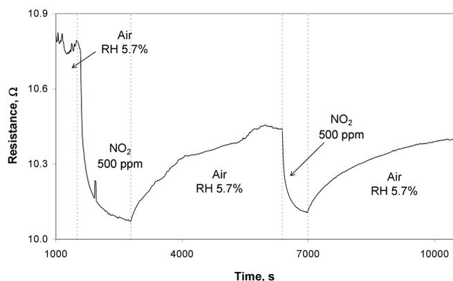
Fig. 16. Sensitivity of the sensor structure with graphene to the presence of  $\text{NO}_2$  in the atmosphere of synthetic air (temperature of the structure  $50^\circ\text{C}$ , humidity RH about 5%)
