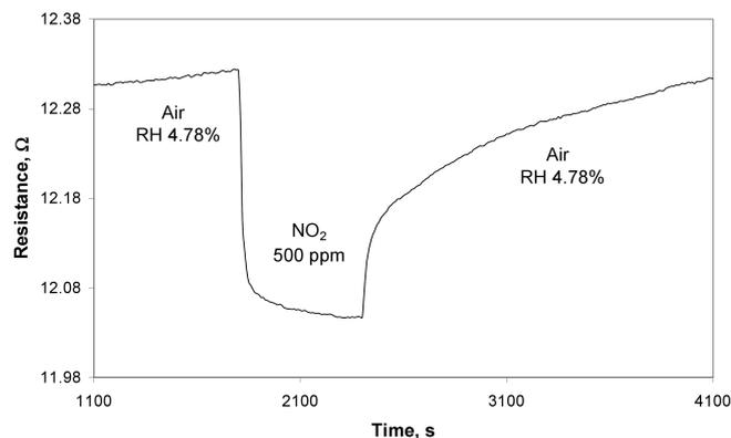
Fig. 18. Sensitivity of the sensor structure with graphene modified by a 3 nm Pd layer to the presence of  $\text{NO}_2$  in the atmosphere of synthetic air (temperature of the structure  $120^\circ\text{C}$ , humidity RH about 5%)
