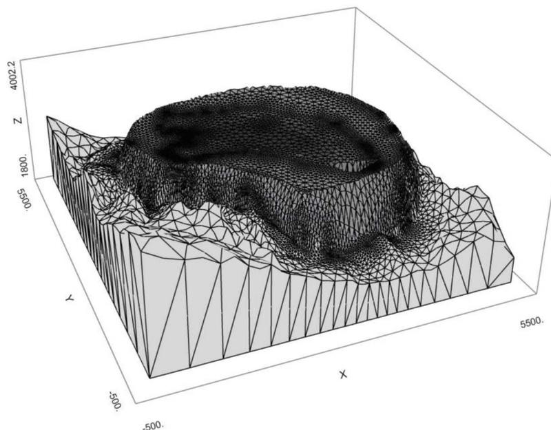
Fig. 2. View of spatial finite element mesh for the "Żelazny Most" landfill.
