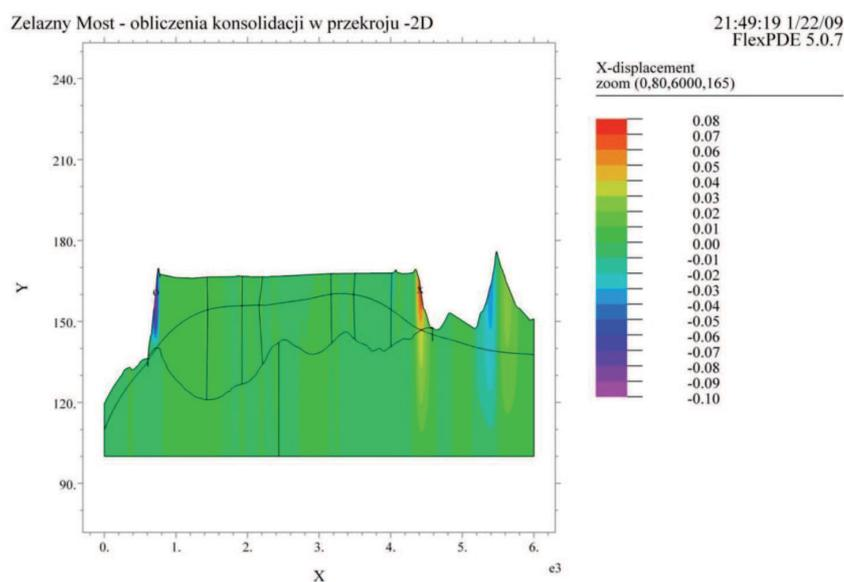
Fig. 8. Graph of horizontal displacement.
