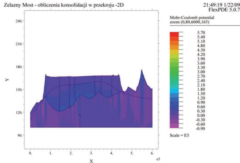
Fig. 12. Results for 2D model – Mohr-Coulomb potential.
