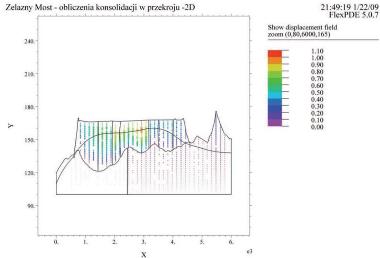
Fig. 7. Vector field of movements of material from the landfill.
