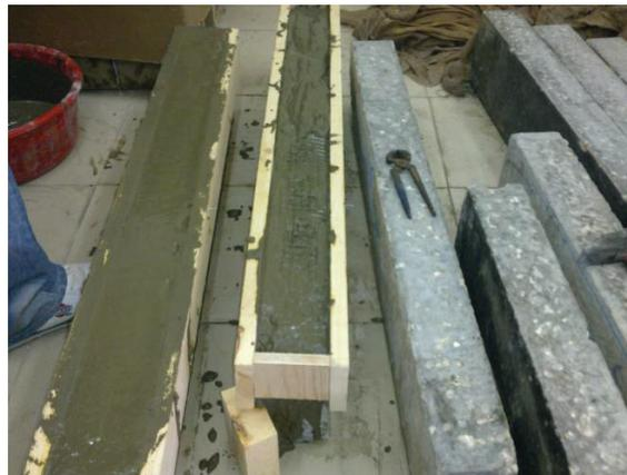
Fig. 6. Cement mortar C1S or C2S used to fix the strengthening layer
