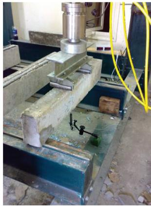
Fig. 8. Testing frame and loaded beam
