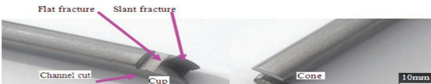
(f) Fractured experimental specimen of the wire with channel-shaped notch.
