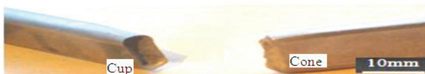
(f) Fractured experimental as-received wire specimen
