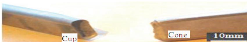
(f) Fractured experimental as-received wire specimen
