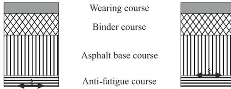
Fig. 4. Schemes of fatigue crack initiation in pavement structure with anti-fatigue course
