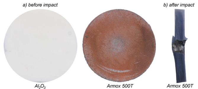
Fig. 8. Panel components before and after impact
