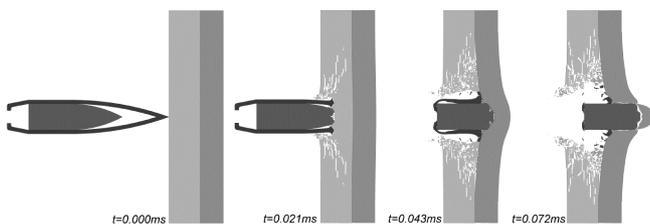
Fig. 7. Perforation of optimal panel
