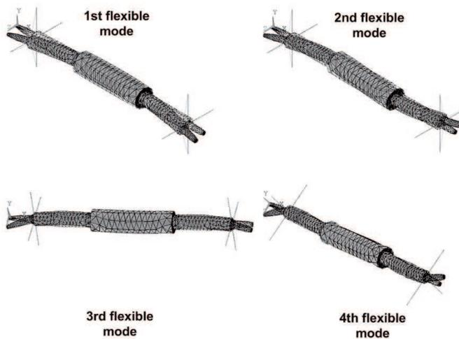
Figure 6. Flexible modes of the AMB flexible rotor.
