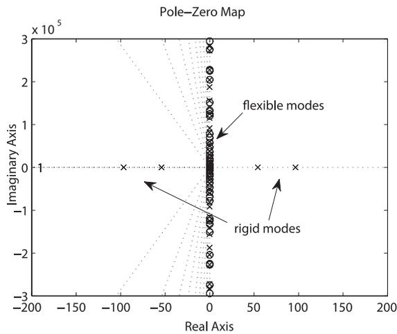
Figure 5. Pole distribution of the flexible rotor in AMB.
