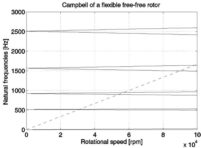
Figure 3. Campbell diagram of the free-free rotor.
