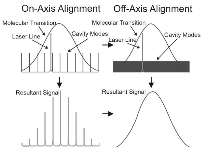
Fig. 5. Mode spectra on-axis alignment and off-axis one
