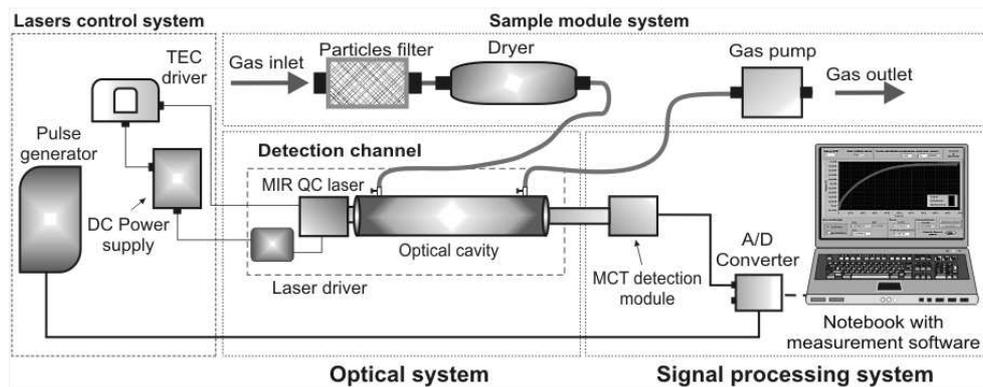
Fig. 15. Block diagram of the MIR sensor
