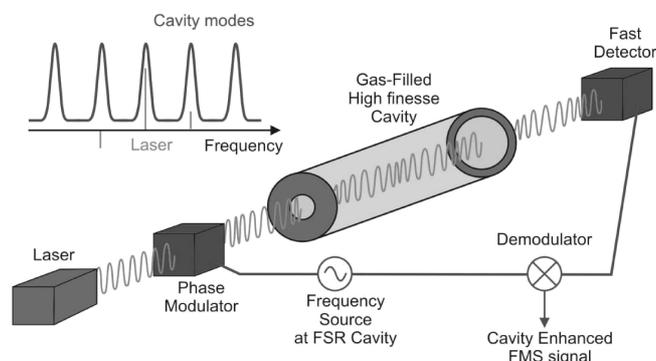
Fig. 4. Idea of the NICE-OHMS detection system
