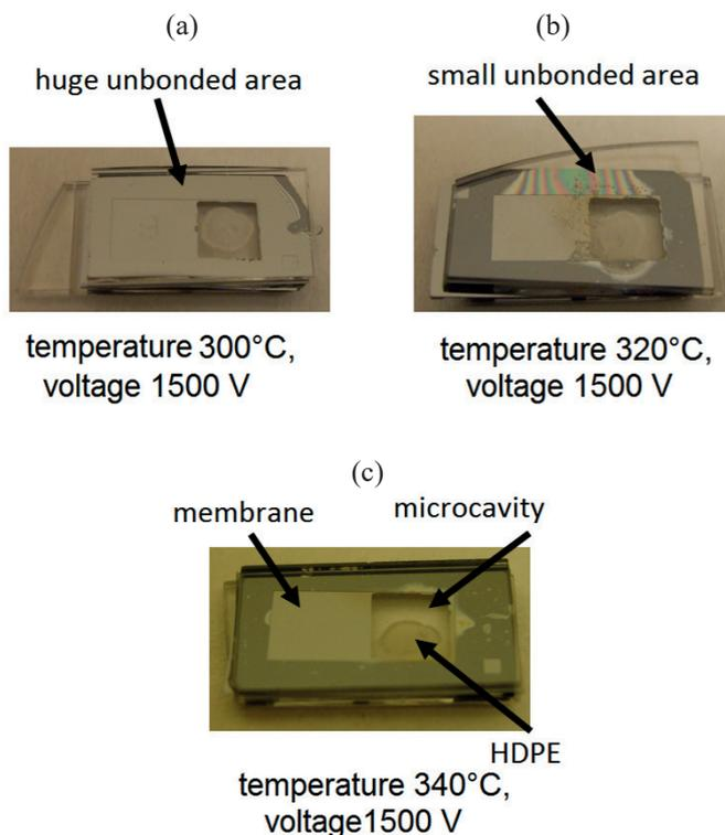
Fig. 6. The sealing polymer in the form of micropellets in silicon-glass micro-inches for the parameters of the process: (a)  $300^{\circ}\text{C}$ ,  $1500\text{ V}$  – no connection; (b)  $320^{\circ}\text{C}$ ,  $1500\text{ V}$  – partial connection; (c)  $340^{\circ}\text{C}$  and  $1500\text{ V}$  – good connection
