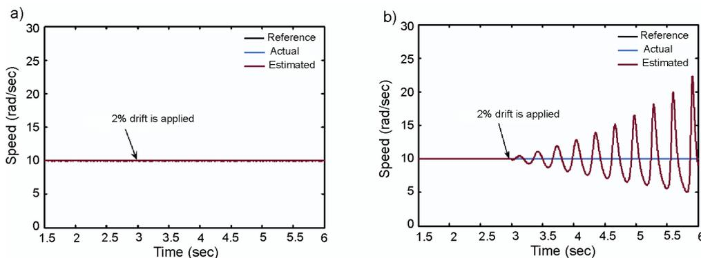
Fig. 12. Response of MRNLAS based speed estimator for integrator drift Problem: (a) RP-MRNLAS
