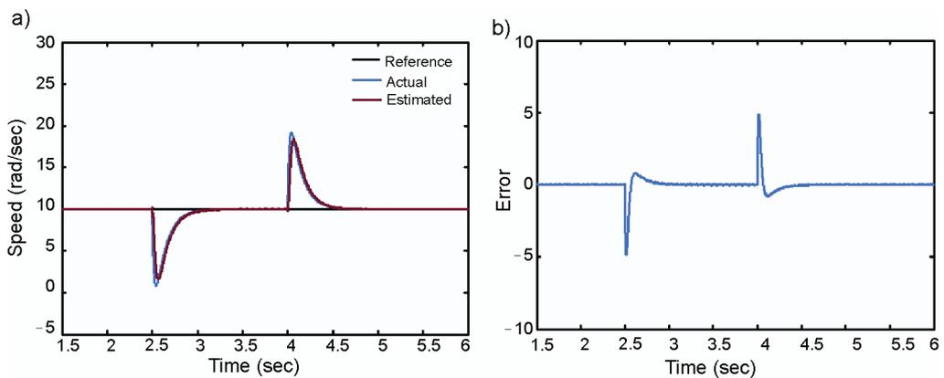
Fig. 6. Performance curves for test condition-3: (a) actual and estimated speed, (b) error between actual and estimated
