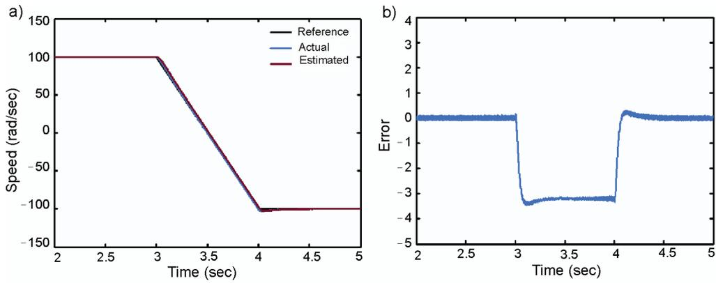
Fig. 7. Performance curves for test condition-4: (a) actual and estimated speed, (b) error between actual and estimated
