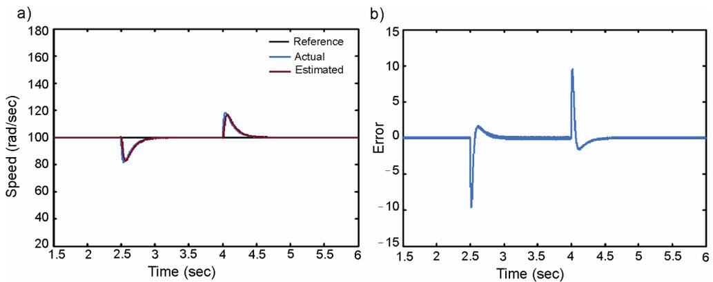
Fig. 5. Performance curves for test condition-2: (a) actual and estimated speed, (b) error between actual and estimated
