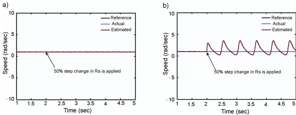
Fig. 11. Rotor speed with large  $R_s$  detuning: (a) RF-MRNLAS (b) RP-MRNLAS
