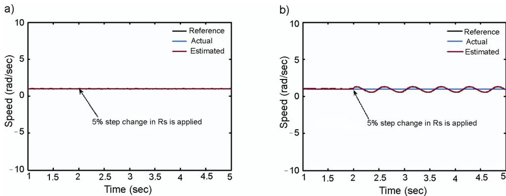
Fig. 10. Rotor speed with slight  $R_s$  detuning: (a) RP-MRNLAS (b) RF-MRNLAS
