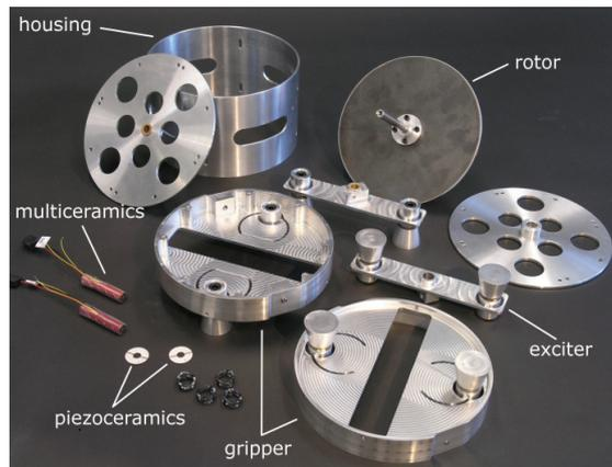
Fig. 12. Disassembled prototype hybrid piezoelectric motor [6]
