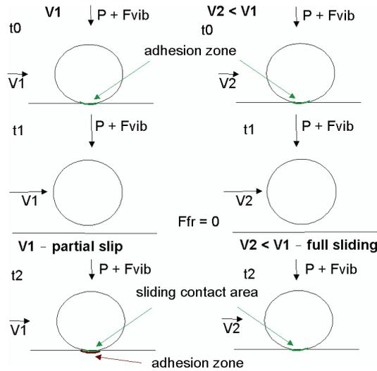
Fig. 4. Illustration of the electroactive lubrication principle applied in the hybrid piezoelectric motor:  $V_1, V_2$  – velocities of the moving body,  $t_0$  – full adhesion interval;  $t_1$  – separation interval;  $t_2$  – partial or full slip interval;  $P$  – static normal force;  $F_{vib}$  – normal force due to vibration;  $F_{fr}$  – friction force
