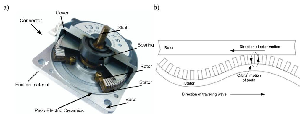
Fig. 2. Traveling-wave piezoelectric motor based on resonance structure:
