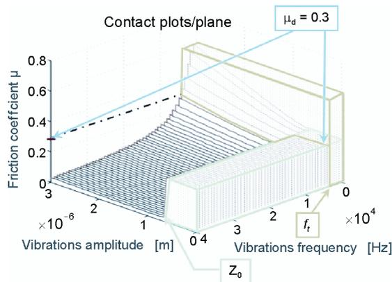
Fig. 5. Evolution of the friction coefficient as a function of the amplitude and frequency of vibrations for the discretized contact;  $Z_0$  – minimal amplitude of vibrations;  $f_t$  – minimal frequency of vibrations;  $\mu_d$  – selected dynamic friction coefficient
