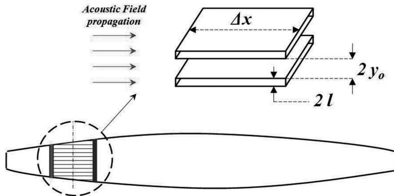
Fig. 7. Geometrical parameters of a parallel plate stack
