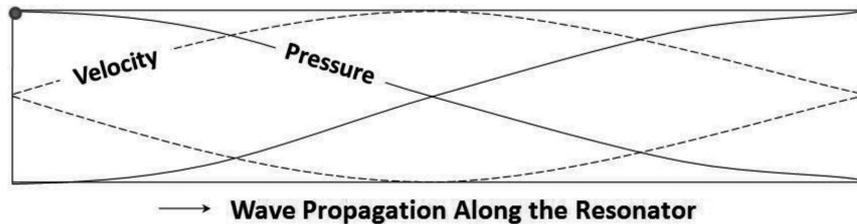
Fig. 3. Variation of pressure and velocity amplitudes along the resonator of a  $\lambda/2$  standing wave engine. The circle at the top left corner denotes the pressure anti-node nearest to the stack's location
