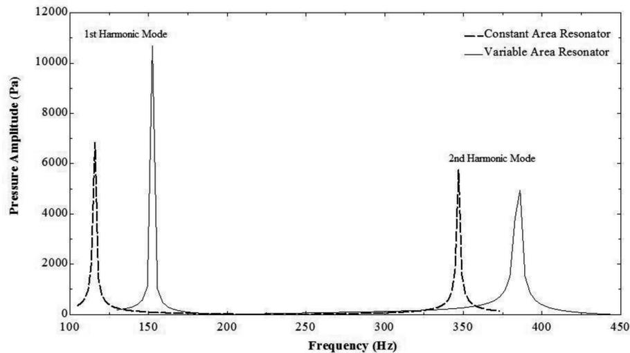
Fig. 1. Response of pressure amplitude to frequency variation for constant and variable area tubes of the same average diameter. The curve is drawn at a pressure of 1 bar using atmospheric air as the working fluid (Abdel-Rahman 2009)
