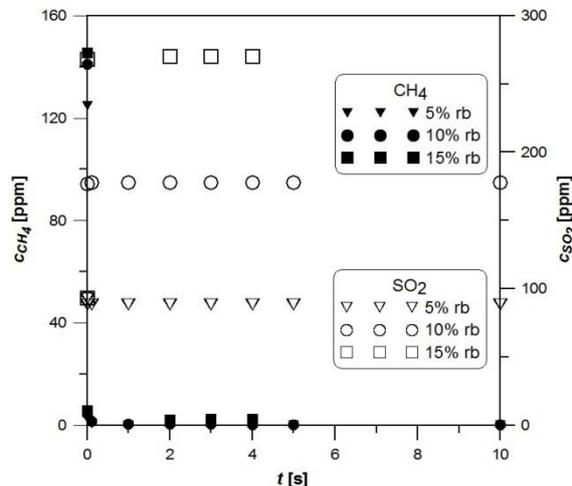
Fig. 9. Concentration of CH<sub>4</sub> and SO<sub>2</sub> as a function of residence time and reburning gas addition
