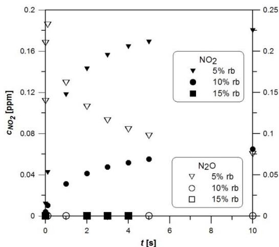
Fig. 8. Concentration of NO<sub>2</sub> and N<sub>2</sub>O as a function of residence time and reburning gas addition
