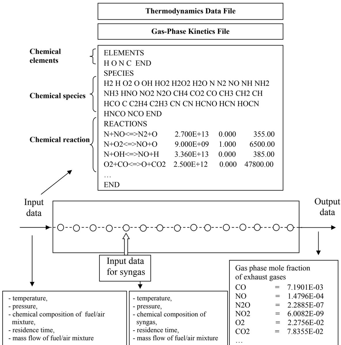
Fig. 1. A scheme of numerical modelled combustion chamber
