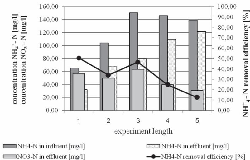
Fig. 1. Nitrogen compounds concentration and ammonia oxidation effectiveness measured for MBR bioreactor during the experiment;  $\text{NO}_2^-$  concentrations in the effluent not shown due to a very low values obtained
